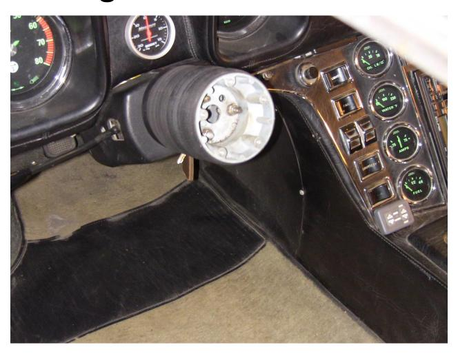
Hub Spacer Removed – 22mm socket Remove the 2 screws in the shroud and bag the screws (left is different than the right)
