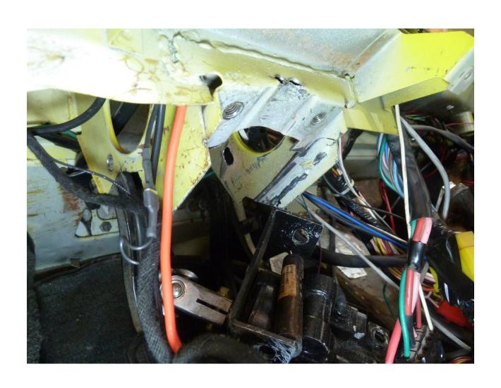
Box Rounded by drilling 2 holes..Cutting between them with air jigsaw. Pipe & Hammer to contour the top section up.
